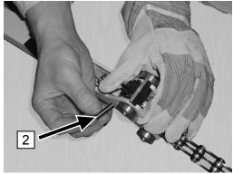
3. Close the locking flap again with a screwdriver. The locking pin secures itself upon closing of the locking flap.
