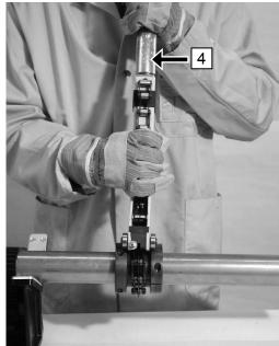
3. Add tension to the chain with even levering motions of at least 90° until the cutting wheels press into the pipe wall.
